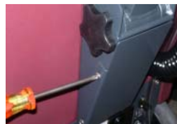
Screw the cover back with the 4 screws.
